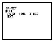
This is used to select the IR-CUT Filter operation mode.
